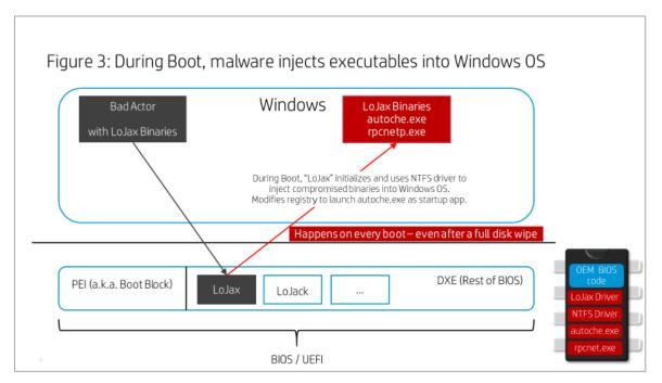
After installing these two files on the disk, the LoJax driver also makes a modification to the registry to automatically run autoche.exe, instead of autochk.exe on every boot. The one letter difference between the two file names (autoche.exe vs. autochk.exe) can be difficult to detect by a person visually inspecting the registry.
